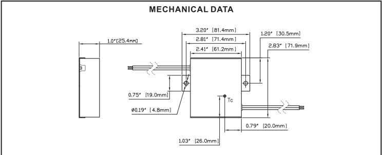
Where: L = Length, W = Width, H = Height, Tolerance=±0.02"
