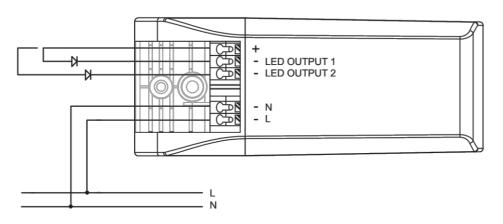
Note: Only connect LEDs to one output at the same time.
