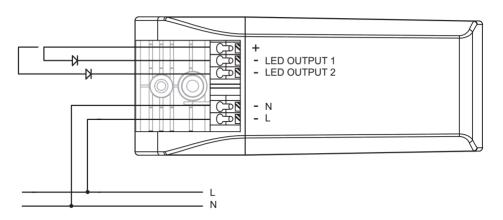
Note: Only connect LEDs to one output at the same time.
