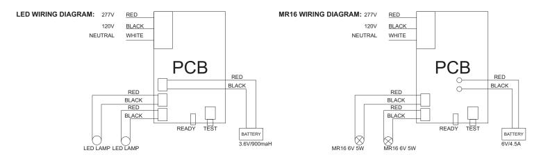
NOTE: UNUSED LEAD TO BE PROPERLY INSULATED WITH WIRE NUT OR OTHER APPROVED METHOD
