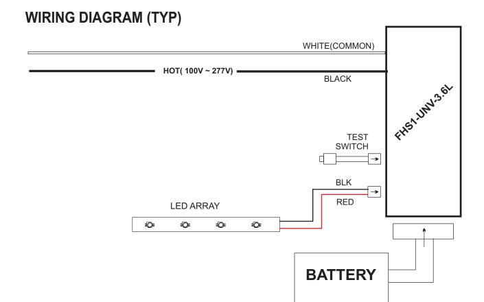
IMPORTANT: Do not connect battery until fixture is installed
