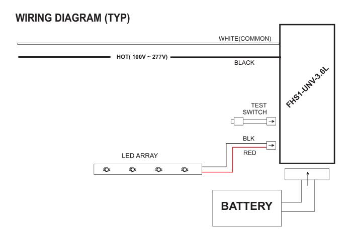
IMPORTANT: Do not connect battery until fixture is installed
