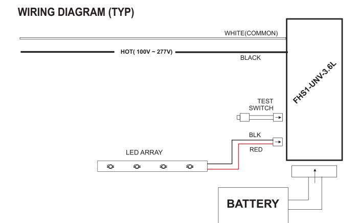
IMPORTANT: Do not connect battery until fixture is installed
