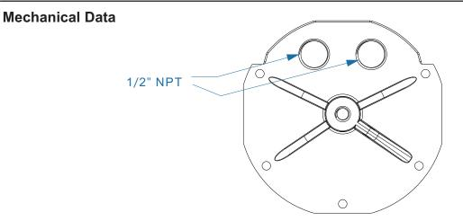
**Overall Dimensions** 5.47" Diameter (139mm) 6.80" Height (173mm)
