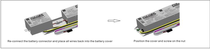
STEP 3: Re-assemble the battery cover
