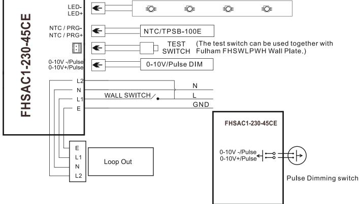
**Description:** The Fulham FHSWLPWH Wall Plate can be used when remote mounting the Lighted Push Button Test Switch (LPBTS) next to the fixture, on the wall or in any location within the maximum remote mounting distance (15 meters) of the Lighted Push Button Test Switch (LPBTS).
