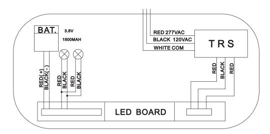
WARNING: Unused wires must be capped using enclosed wire nuts.
