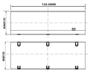
Note: All Dimensions are in mm. Tolerance=±0.5mm
