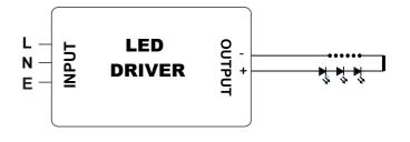
Installation Instructions: Keep proper ventilation around the LED Driver and do not stack any object on it. Also a 10-15 cm clearance must be kept when the adjacent device is a heat source. Do not exceed the declared Hot spot temperature(Tc max) under any circumstances.
