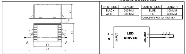
Installation Instructions: Keep proper ventilation around the LED Driver and do not stack any object on it. Also a 10-15 cm clearance must be kept when the adjacent device is a heat source. Do not exceed the declared Hot spot temperature(Tc max) under any circumstances.
