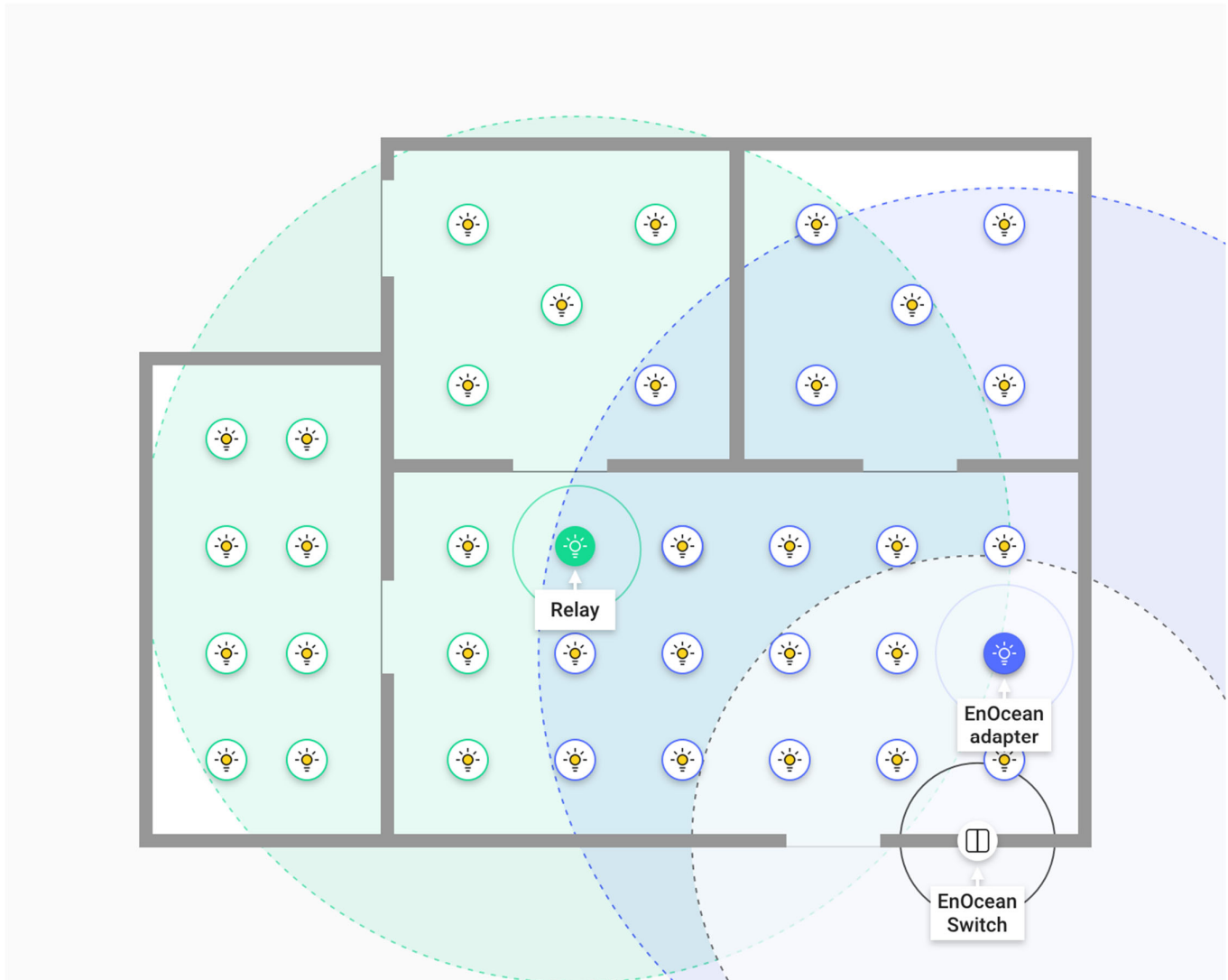
fig.1 Correct placement of Relays and EnOcean adapter options
