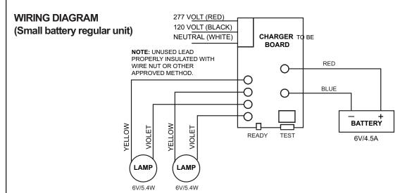
**WARNING:** Unused wires must be capped using enclosed wire nuts.
