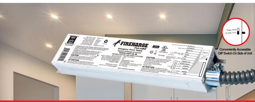
The Fulham FireHorse FHUPS1-UNV-12L-SD is a 12 Watt Micro-Inverter / Emergency Power Supply that delivers power to any fixture in emergency mode at 12W for 90 minutes (it can be programmed down to 6W for 160 minutes, or with tiered selections in between).
