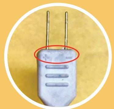
Identify the polarity on the programming cable.
